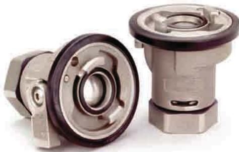
The Eaton FD83 is designed for fluid transfer and electronics cooling applications where full flow, fluid compatibility and safety are essential. The FD83 identical halves include two interlock features to eliminate spills and ensure maximum safety. Valves cannot be opened until the coupling halves are mated and coupling halves cannot be disconnected until both halves are closed. The FD83 coupling system can be used in a wide variety of low pressure industrial applications.
